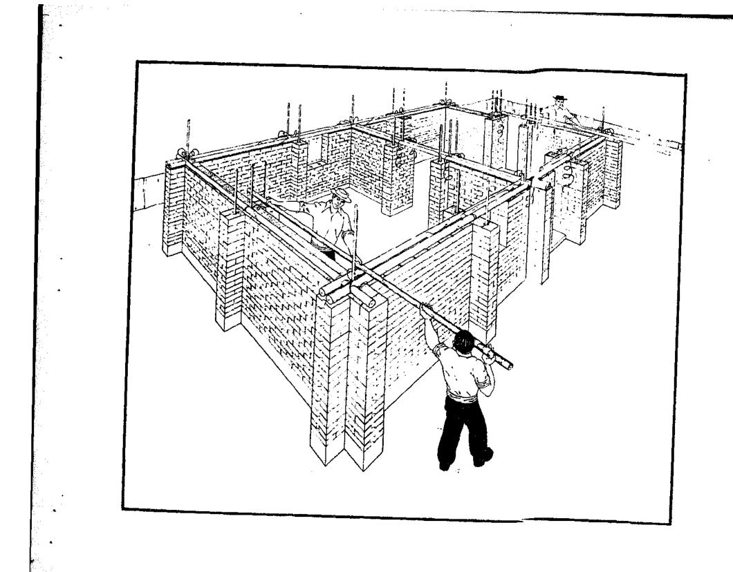
In this drawing, the <u>maestro</u> is tying the collar beam down to the wall.
