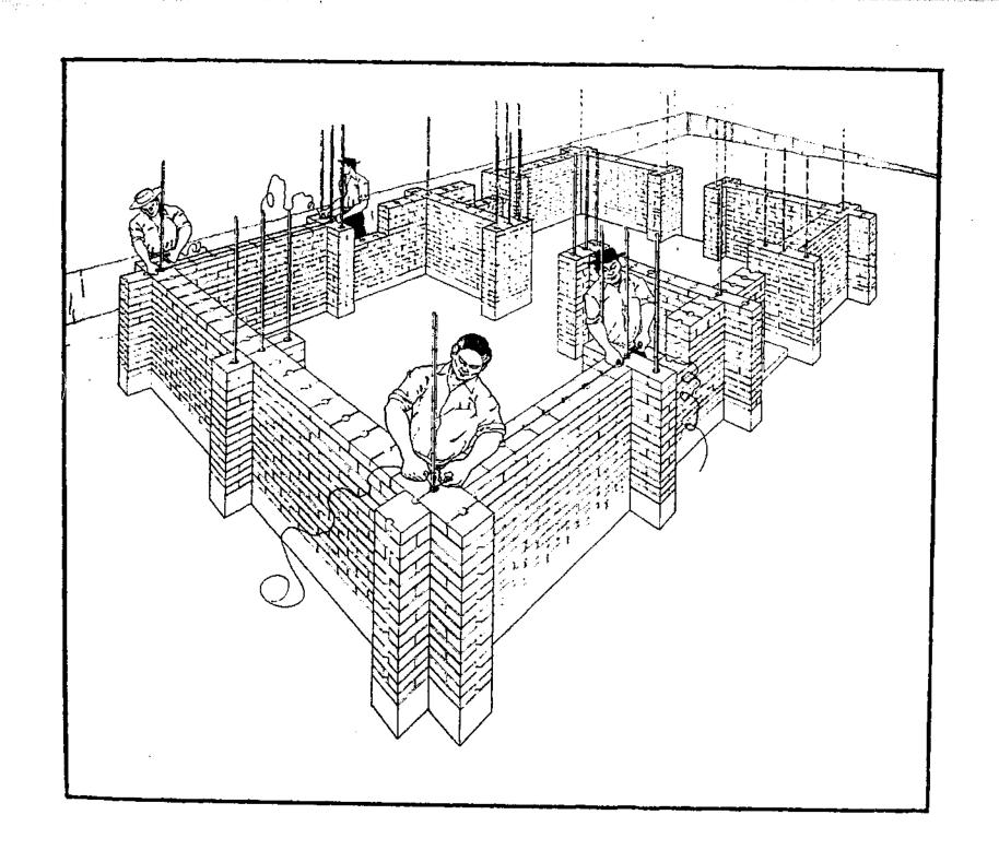
In this drawing, the <u>maestro</u> has put a layer of adobe over one of the wires and is pulling the end up along the rod.
