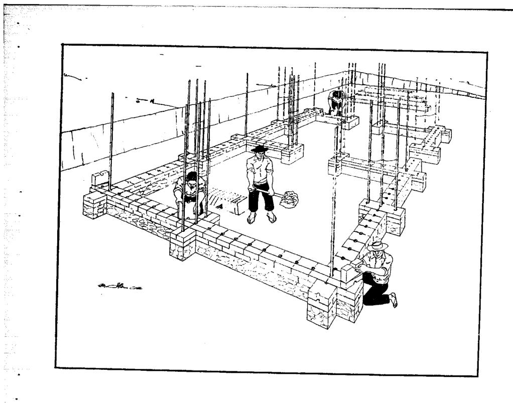
This is a drawing of how to make a mocheta (pilaster).
