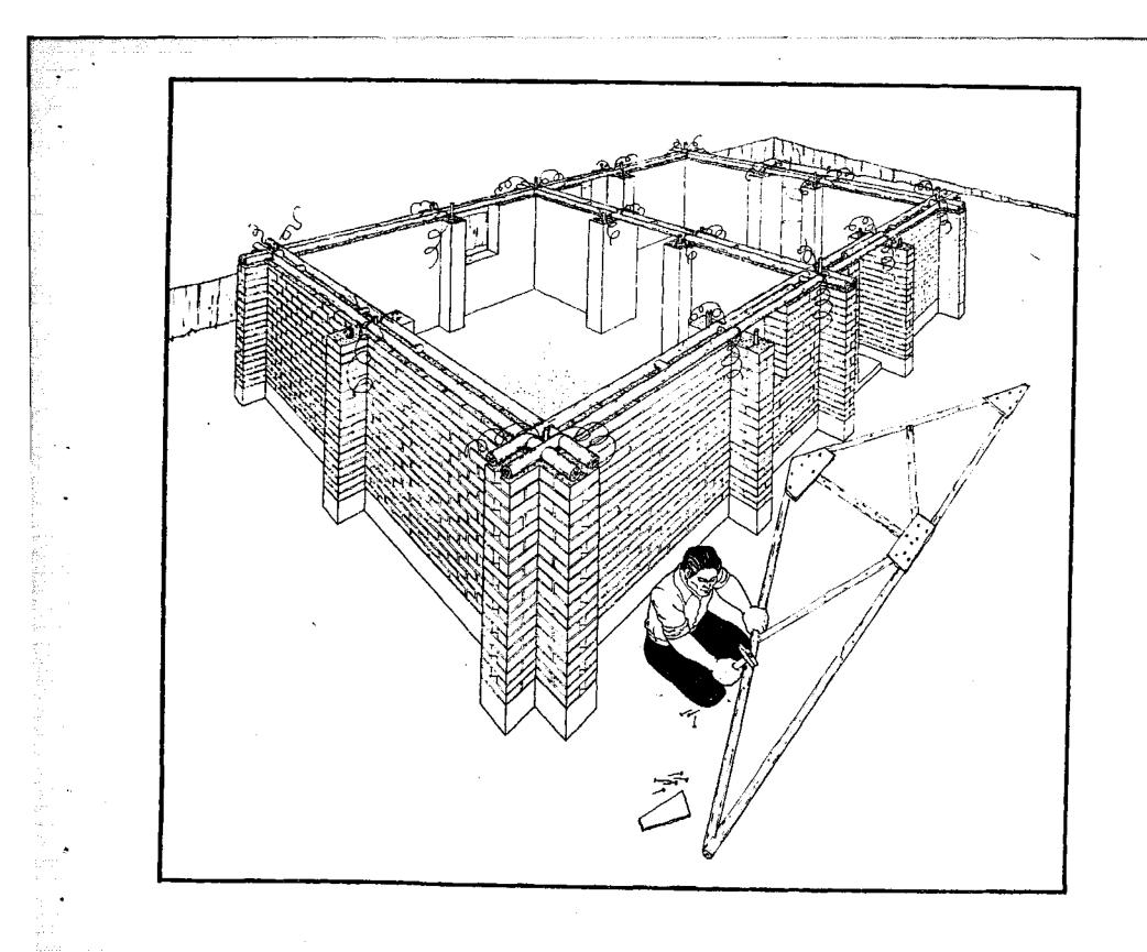
In this drawing, the men are fastening the truss to the collar beam.
