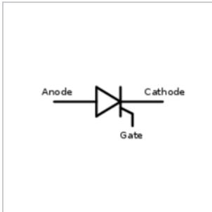
Silicon-controlled rectifier (SCR)
