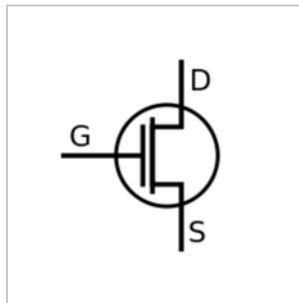
Metal-Oxide-Semiconductor Field-Effect Transistor
