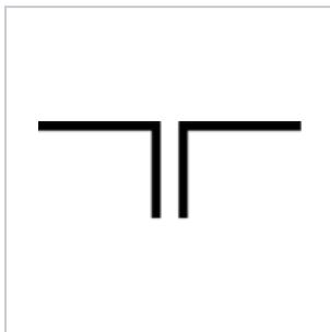
IEC-style dipole antenna
