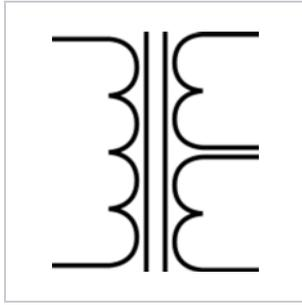
Transformer with two secondary windings
