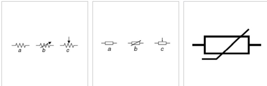
(a) American-style resistor, (b) rheostat (variable resistor), and (c) potentiometer
