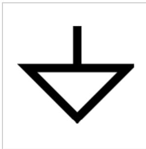
Signal/Low noise ground (GND) symbol
