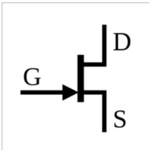
N-channel junction gate field-effect transistor (JFET)
