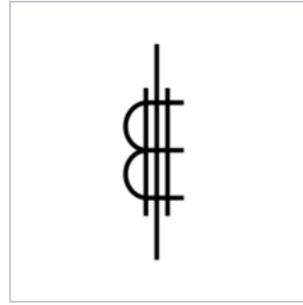
Zero-Sequence Current Transformer (ZSCT) (a.k.a. window-type current transformer)
