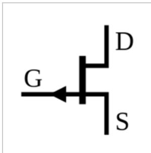
P-channel junction gate field-effect transistor (JFET)
