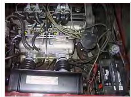
Chevrolet Cosworth Vega engine showing Bendix electronic fuel injection (in orange).
