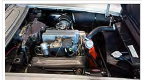
A 1959 Corvette small-block 4.6 litre V8 with Rochester mechanical fuel injection
