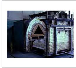
A Catenary Arch kiln used for firing high temperature electron tube grade aluminium oxide ceramics
