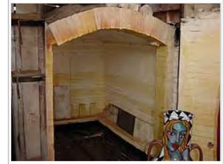
An empty, intermittent kiln. This specific example is a "car kiln"; the base is on wheels and has been rolled out of the kiln - this facilitates loading and unloading the kiln
