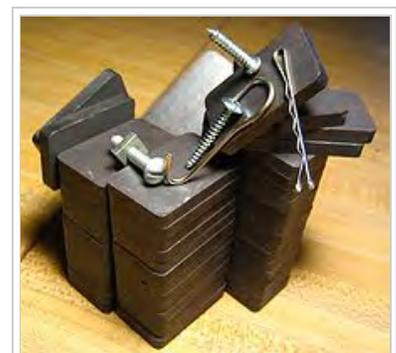
A stack of ferrite magnets
