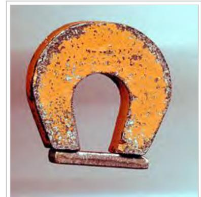
A "horseshoe magnet" made of alnico, an iron alloy. The magnet, made in the shape of a horseshoe, has the two magnetic poles close together. This shape creates a strong magnetic field between the poles, allowing the magnet to pick up a heavy piece of iron.
