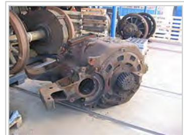
Nose-suspended traction motor for a Czech ČD class 182 locomotive
