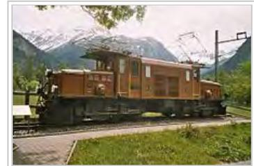
Swiss Rhaetian Railway Ge 6/6 I Krokodil locomotive, with a single large traction motor above each bogie, with drive by coupling rods.
