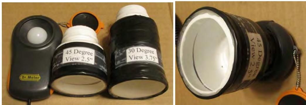
The 45 degree viewing light shield above measured 2.25" and the 30 degree angle of view measured 3.5" high with an added .25" to the sensor this gives what was marked in the pictures above as 2.5" and 3.75".
