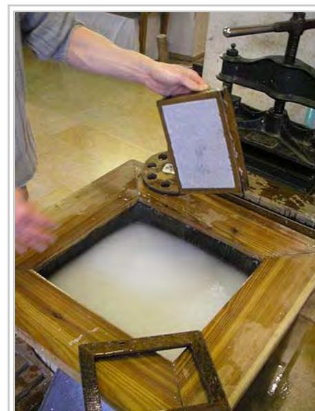
A sheet of fibres which were just collected from the liquid suspension with the screen. The next steps are to press it and to dry it.
