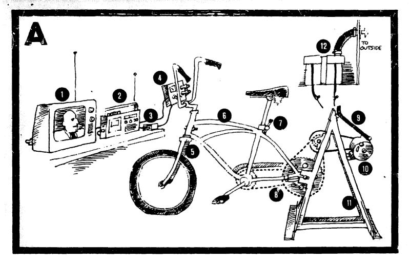
The prototype described here was built by the North Shore Ecology Center to find correct gear ratios for electric generation and for other foot-power mechanical devices. Possible applications might be: garden mulcher, flexible shaft drill, grinder, circular saw, air or water pump, etc.
