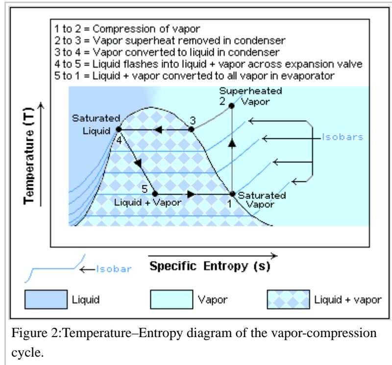
Figure 2: Temperature-Entropy diagram of the vapor-compression cycle.
