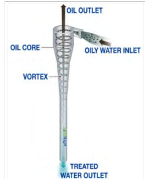
Centrifugal forces in a hydrocyclone for oily water separation
