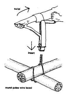
Fig. 5.2 Diagram of the Delft wire lacing tool.
