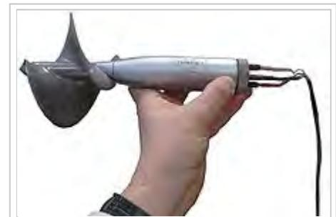
A propeller-type current meter as used for hydroelectric turbine testing.
