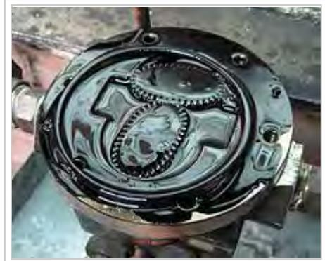
A positive displacement flowmeter of the oval gear type. Fluid forces the meshed gears to rotate; each rotation corresponds to a fixed volume of fluid. Counting the revolutions totalizes volume, and the rate is proportional to flow.
