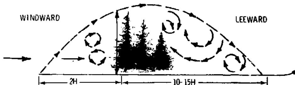
FIGURE 4.9. Airflow Near a Shelterbelt<sup>(12)</sup>
