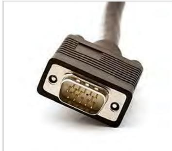
A *male* D-Subminiature connector which serves as a *plug*. The pins make this connector male; the surrounding shield does not change that.
