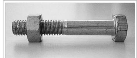
*Female* nut threaded onto a *male* bolt
