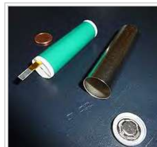
Cylindrical Panasonic 18650 lithium-ion battery cell before closing. Several thousand of them form the Tesla Model S battery (see Gigafactory).
