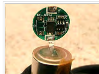
Lithium-ion battery monitoring electronics (over- and discharge protection)
