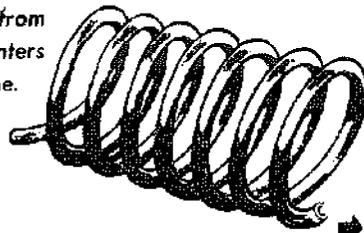
"Metered" liquid refrigerant leaves capillary to go to freezer.
